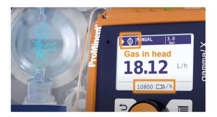
Solenoid diaphragm pump gamma/ X and XL detect air bubbles and react to them with an adapted delivery rate (image source: ProMinent GmbH)
